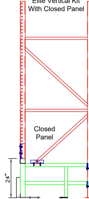
Cut the factory diagonal strut to length for reconnection above repair kit. Fasten to repair kit using (1) Reconnection Angle or Channel and (2) 3/8" diameter Tek screws. Connect strut to reconnection component with supplied fasteners. (All required components are included)
