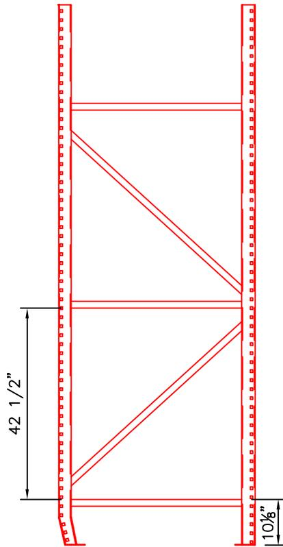
Determine which struts fall below the top horizontal of repair kit. Remove all those struts except for the factory diagonal that intersects with the top horizontal strut on the kit. Measure the intersecting point of diagonal strut and cut at that point. (Follow installation manual for complete Elite installation instructions)
